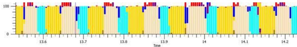
The yellow bars indicate execution of the app's JavaScript—that is, time spent inside the renderer. The beige bars indicate the time spent in DOM layout, and aqua bars indicate actual rendering to the screen. As you can see, when elements are added one by one, there's quite a bit of breakup in what code is executing when, and the kicker here is that most display hardware refreshes only every 10–20 milliseconds (50–100Hz). As a result, there's lots of choppiness in the visual rendering.
