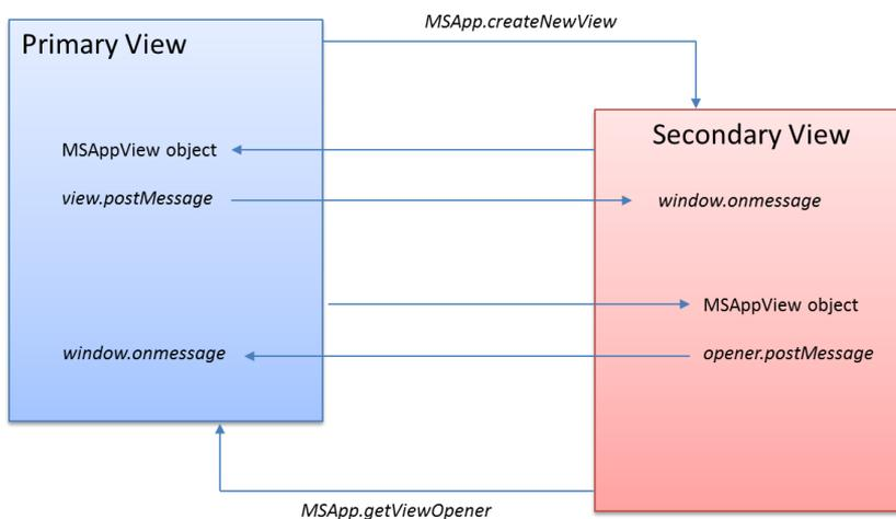
**FIGURE 8-7** A primary view creates a secondary view through `MSApp.createNewView`. The secondary view retrieves a reference to the primary view through `MSApp.getViewOpener`. The result in both cases is an `MSAppView` object whose `postMessage` call sends a message to the other view.
