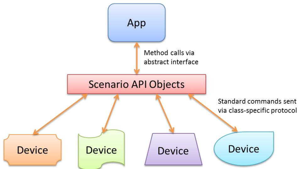
**FIGURE 17-1** Scenario APIs abstract different device classes and the standard commands used to communicate with them. Through that API, an app can work with any number of connected devices that conform to that class.
