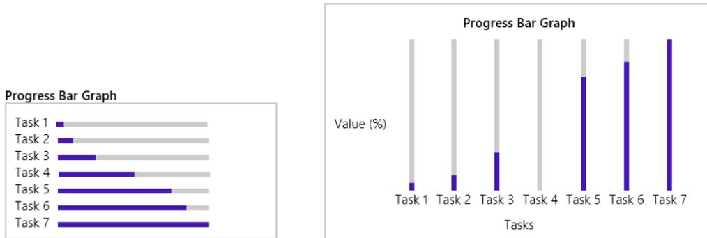
In these cases the whole graph is a `div` (horizontal by default), where the `Repeater` is used inside for the list of tasks to create each bar (`html/scenario4.html`):
