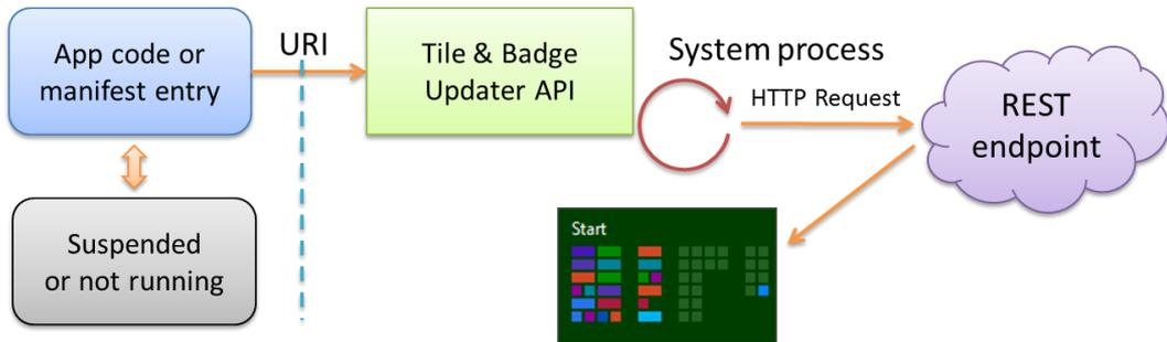
**FIGURE 16-11** Periodic updates for tiles and badges are registered with the system’s tile updater, which will request an update from a given REST endpoint or web service at regular intervals.
