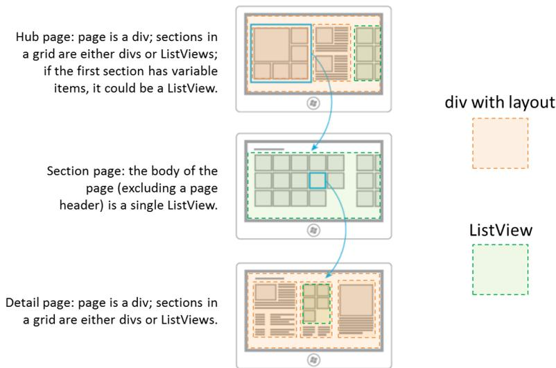
**FIGURE 7-9** Breaking down typical hub-section-detail page designs into `div` elements and `ListView` controls. The Hub control is typically useful for pannable regions that contain different types of sections.
