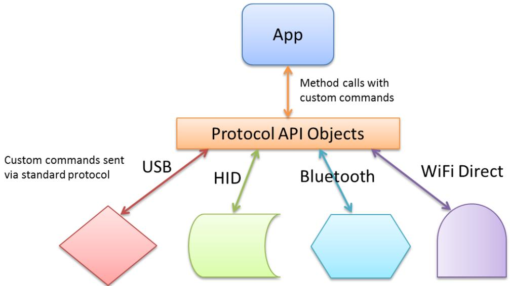
**FIGURE 17-2** Protocol APIs abstract the details of transport protocols—namely USB, HID, Bluetooth, or Wi-Fi Direct—allowing apps to easily send device-specific commands to a wide variety of devices.
