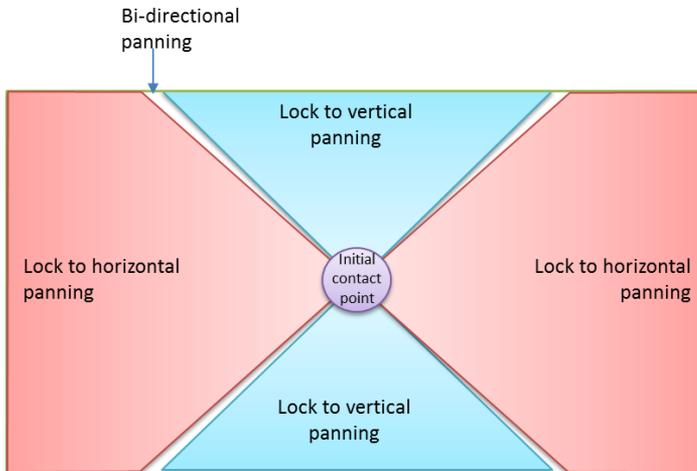
**FIGURE 8-9** The concept of rails, where the white areas indicate regions where the touch point is moved equally along both axes and bi-directional panning can happen. Note that raiing is determined along 45-degree lines from the touch point and has nothing to do with the shape of the region itself.
