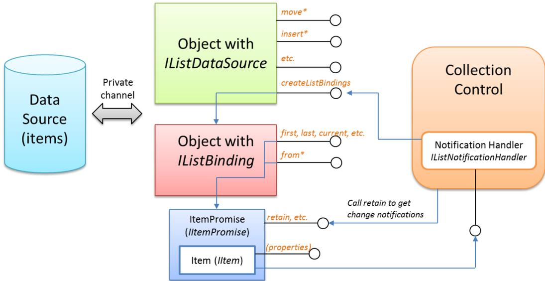
**FIGURE 7-6** The general relationships between a data source, the `IListDataSource` and `IListBinding` interfaces, and a collection control like the `ListView` that uses that data source through those interfaces and provides a notification handler with `IListNotificationHandler` methods.
