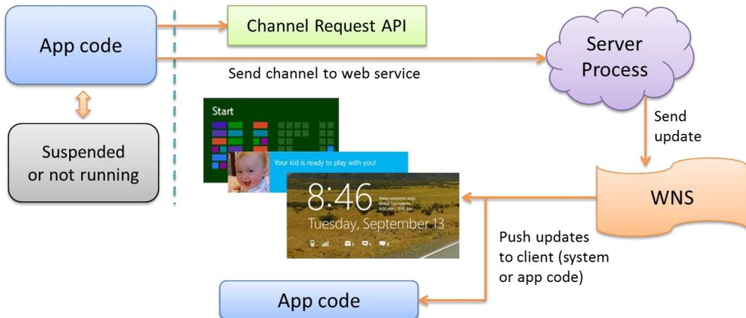
**FIGURE 16-12** Push notifications originate with an always-running server process and are then sent to the Windows Push Notification Service for delivery to specific clients (a specific app on a specific user device) through their registered WNS channels.
