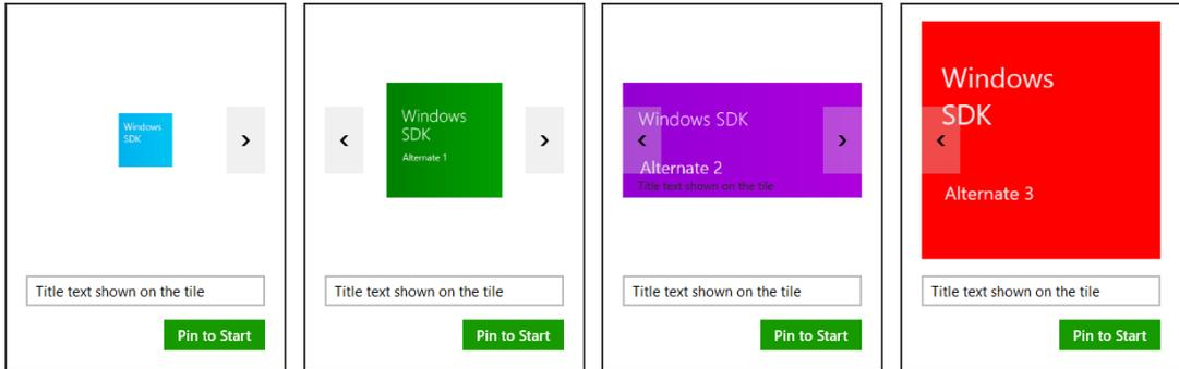
**FIGURE 16-13** Flipping through alternate tile images in the Secondary tiles sample. The blue tiles are the defaults set in the `SecondaryTile` object. The green, purple, and red images, available in all sizes, are set through the `visualElementsRequested` event handler.
